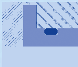
Clamping flange with additional O-ring seal.
